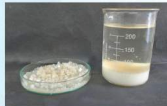
Left: Crystals removed in RO brine treatment Right: Undissolved salt in brine water (@80 °C)
